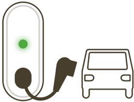
**01** Connect your electric vehicle to the eBox. To do so, plug the cable first into the eBox. When your vehicle is detected, the vehicle link indicator lights up green.
