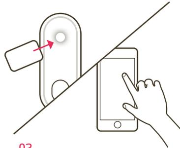
**02** Authenticate the charging process via RFID card or the eCharge+ app. For the latter you will need the charging port number displayed on the front of the eBox. The eBox can also be activated from the backend.
